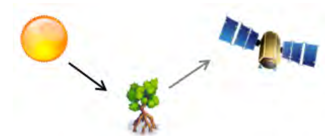
Figure 51 The intensity of the different wavelengths of light reflected from plants to a satellite can be used to assess the health of a plant and in this case, Darwin's mangroves
