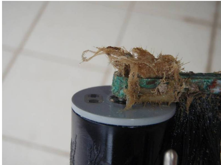
Plate 3-1 Extended deployment logger probe and wiper assembly displaying heavy fouling after 28 days at Howard River mouth
