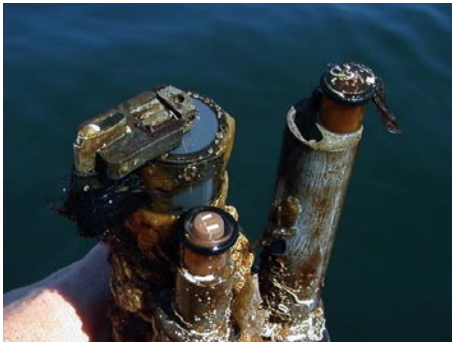
A prototype 6600EDS after continuous deployment for 80 days in Buzzards Bay, MA. The sensor in the foreground is the active DO sensor. The sensor at top-right was used as a non-wiped fouling reference. Note extensive fouling by plant and animal species on the non-wiped sensor.
