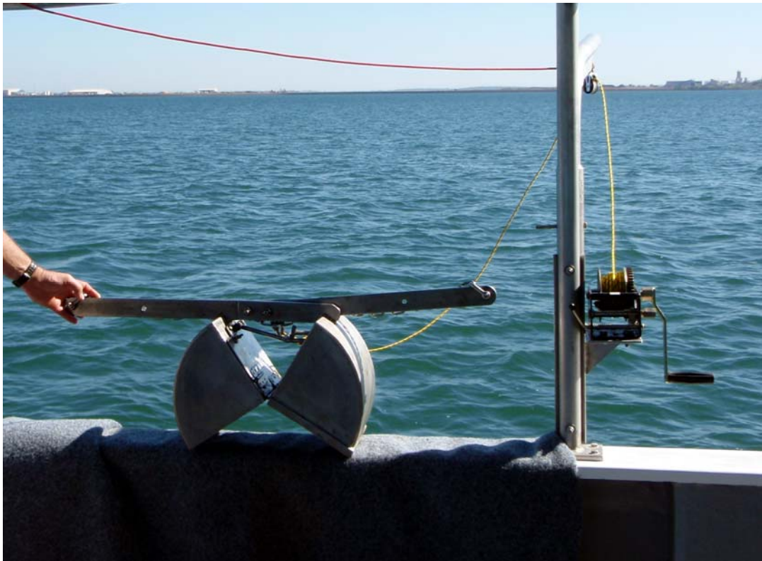
Plate 1 Van Veen Grab used for collecting sediment for infauna determination
