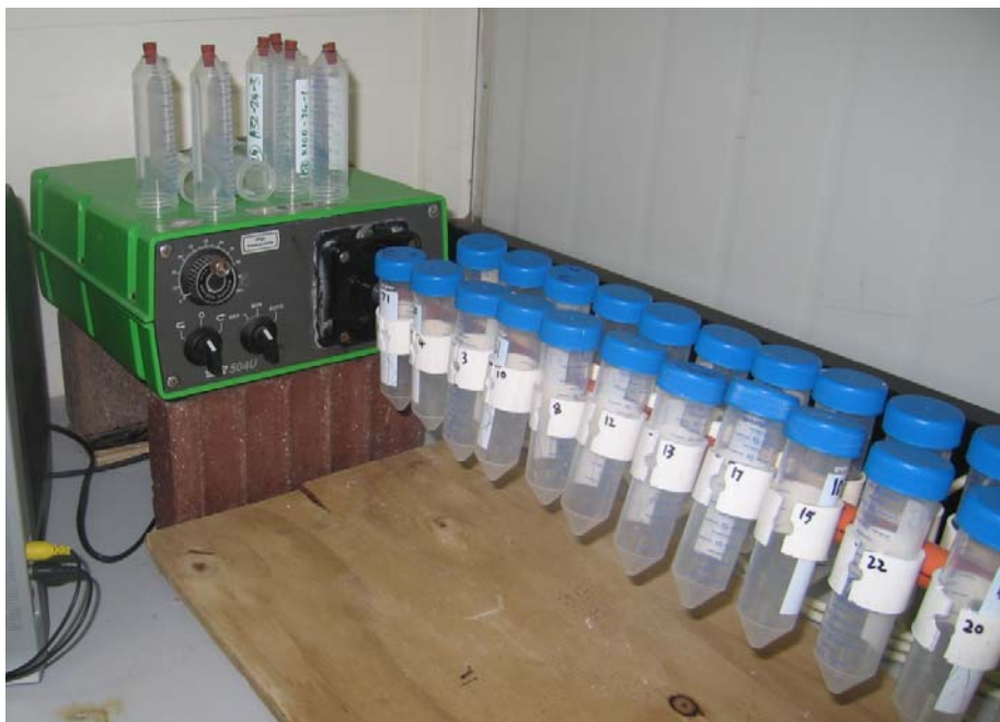
Figure 4: Experimental setup showing the rotating mechanism and 50 mL exposure vials.
