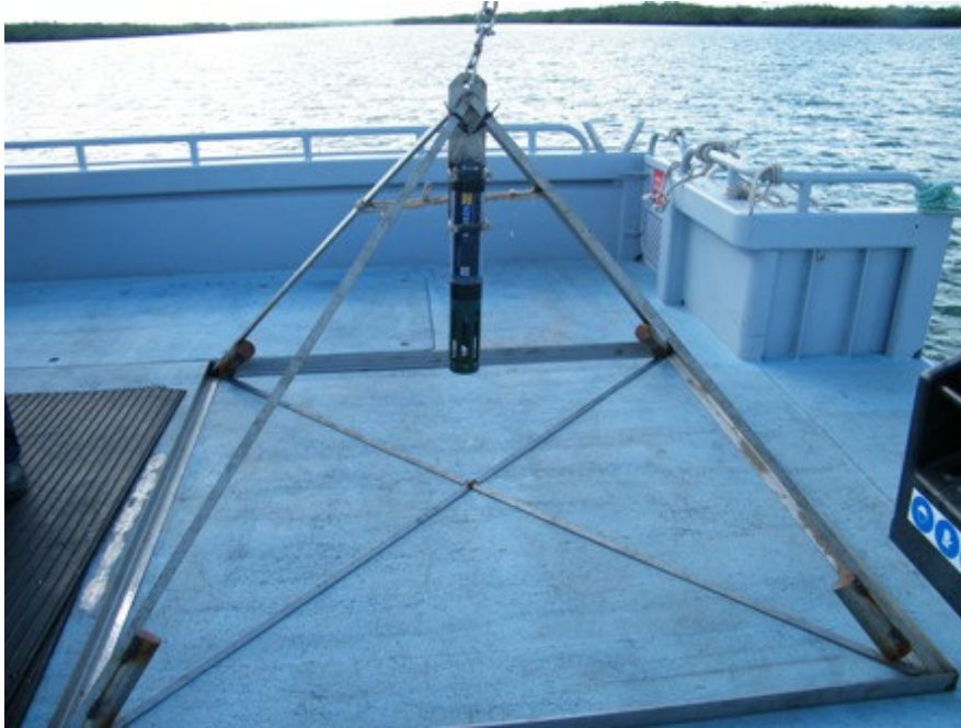
Figure 2-2 Frames used to secure the water quality loggers (with logger in place)
