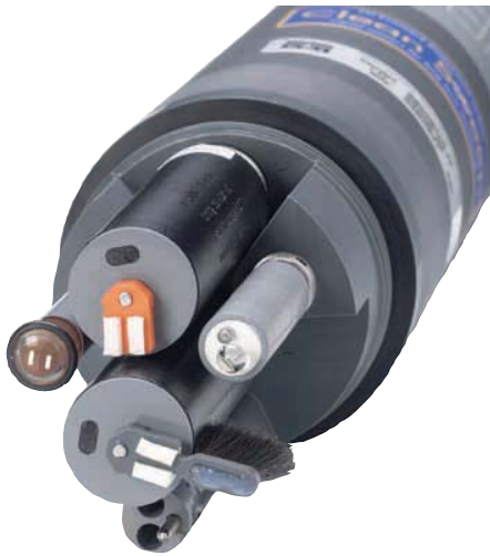
Profile of the 6600EDS depicting (clockwise from bottom) temperature/conductivity, turbidity, Rapid Pulse™ dissolved oxygen, chlorophyll and pH/ORP—all of which (except conductivity) are kept free of fouling by the patented Clean Sweep® universal wiper assembly, as well as individual optical wipers.
