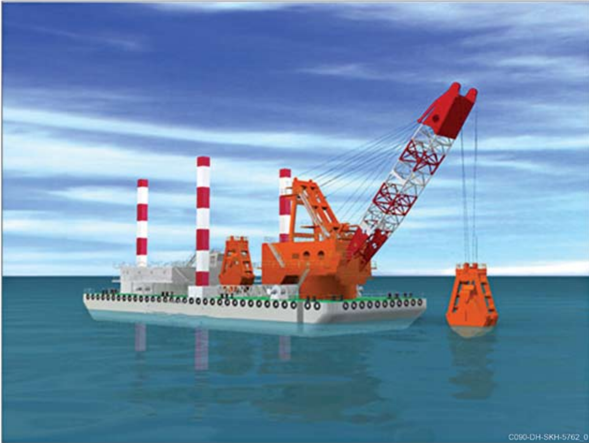
Figure 4-25: Example of a grab dredger
