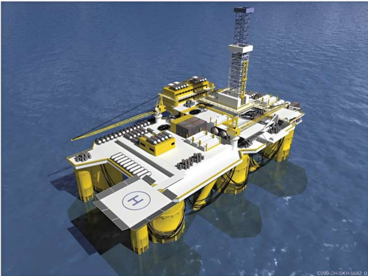
Figure 4-8: Indicative schematic of a semi-submersible drilling rig
