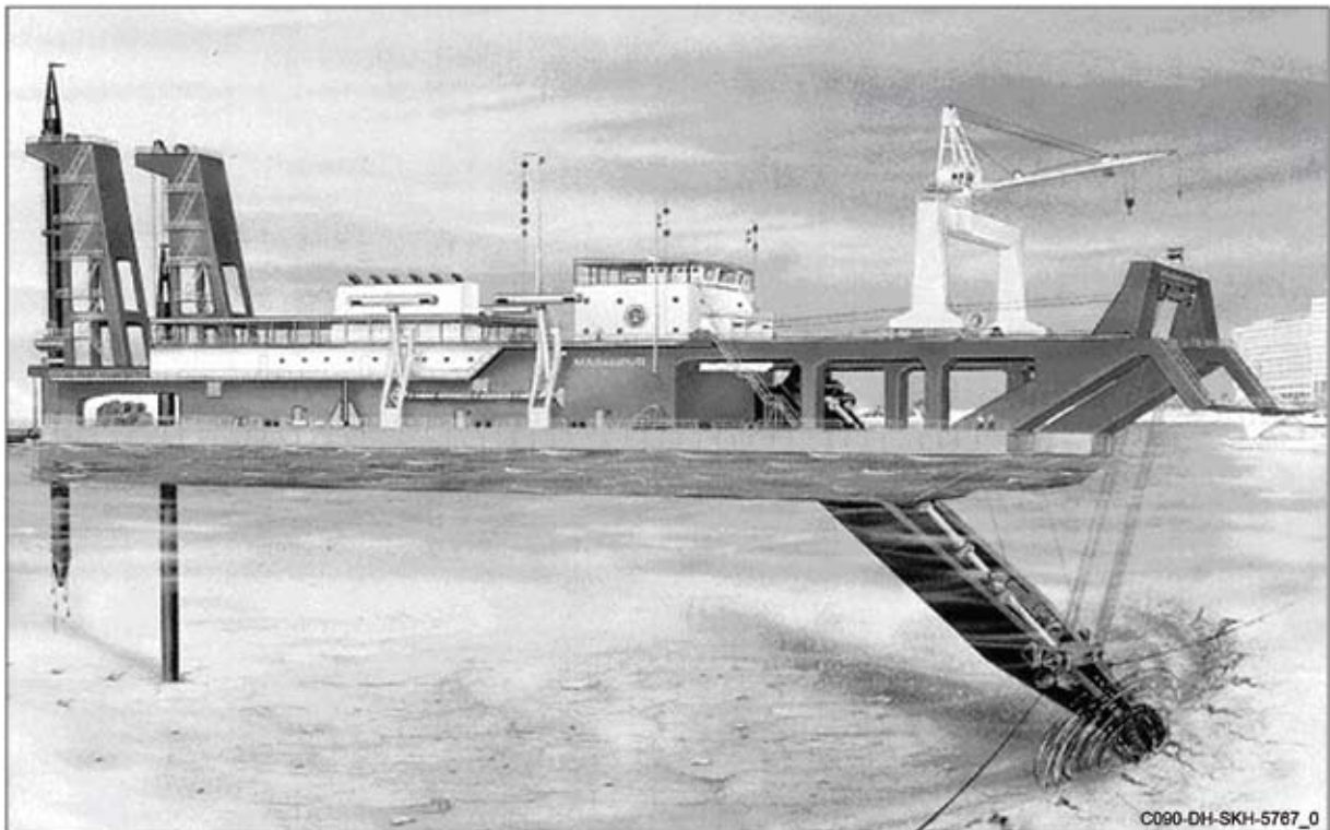
Figure 4-23: Example of a cutter-suction dredger
