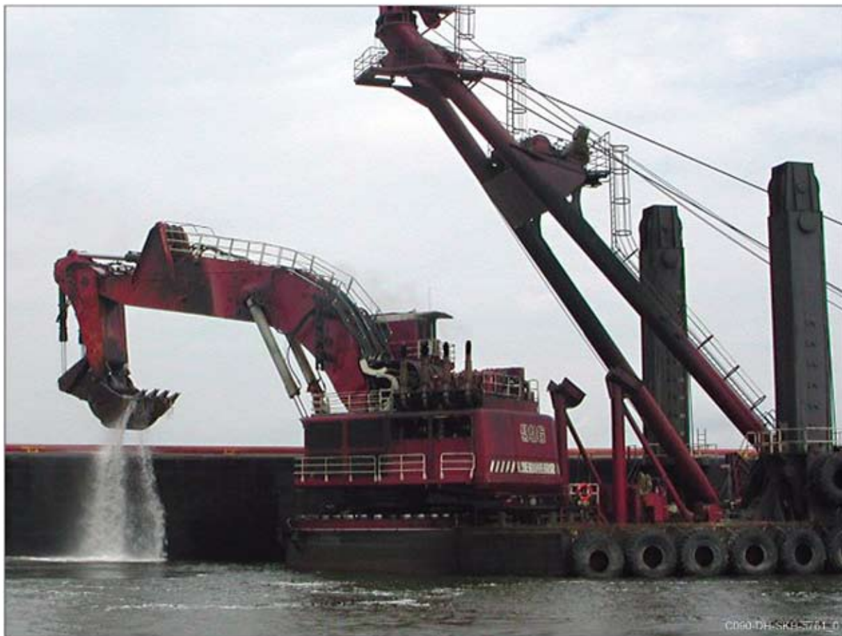
Figure 4-24: Example of a backhoe dredger
