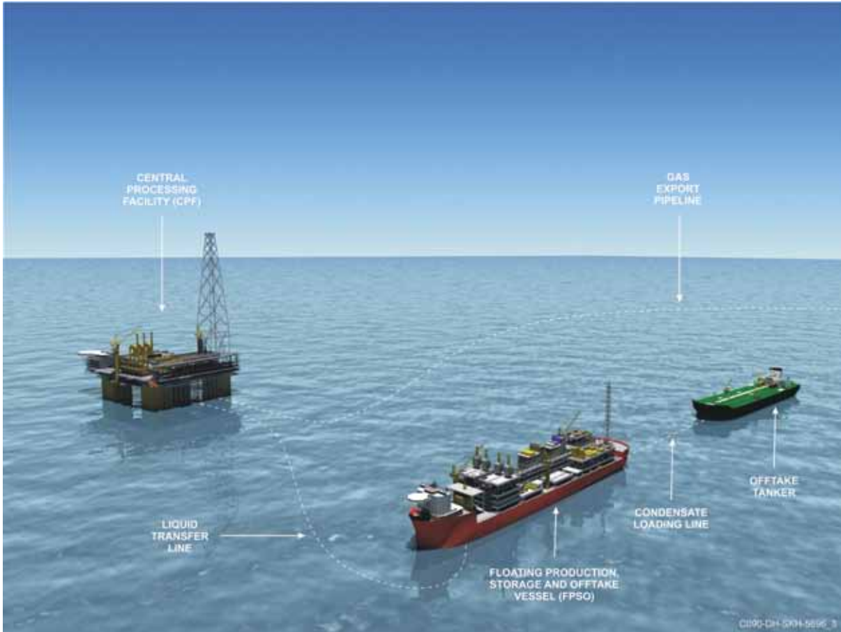
Figure 2-2: Indicative schematic of the offshore floating facilities
