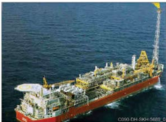
Figure 4-13: Example of an FPSO
