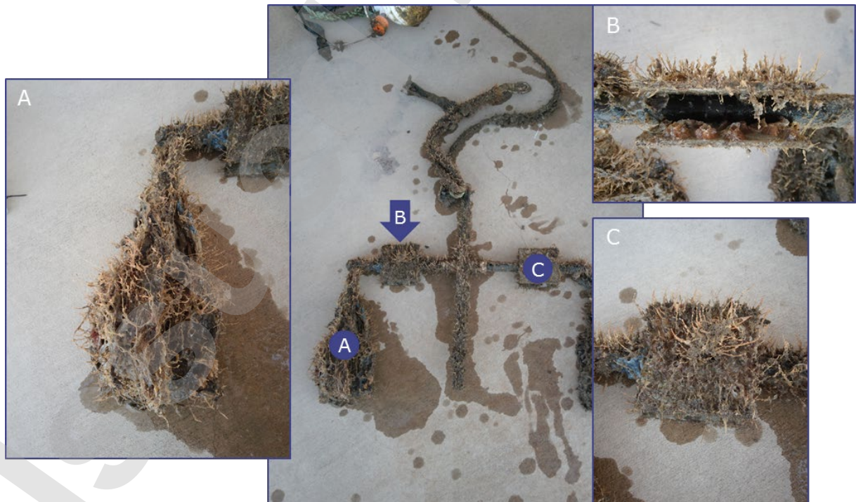
Figure 5-5: Example of monitoring photographs taken during monthly inspection a) rope mop, b) inside the plates and c) plates surface biofouling conditions
